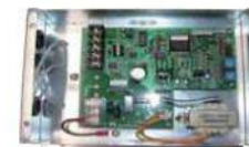
Modbus® Interface TCB-IFMB641TLE
